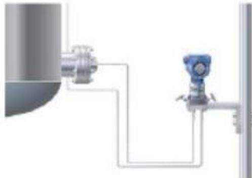
Gambar II.11. *Differential Pressure Level Measurement*
